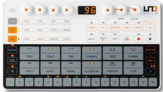
INTERFACE: Aside from the seven rotaries, all controls are flush with the interface with no physical response
