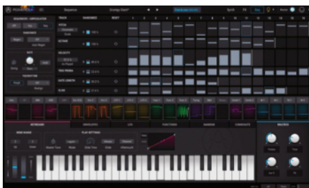
Set the length of each lane independently in the Sequencer/Arpeggiator's Polyrythm mode
