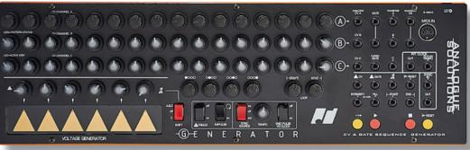
CV/GATE SEQUENCER Three channels of 16 steps that each output an unquantized control voltage (in the range 0-5V)
