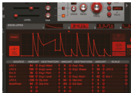
The envelopes can be sustained for holding at a particular point, or looped for LFO-style manoeuvres
