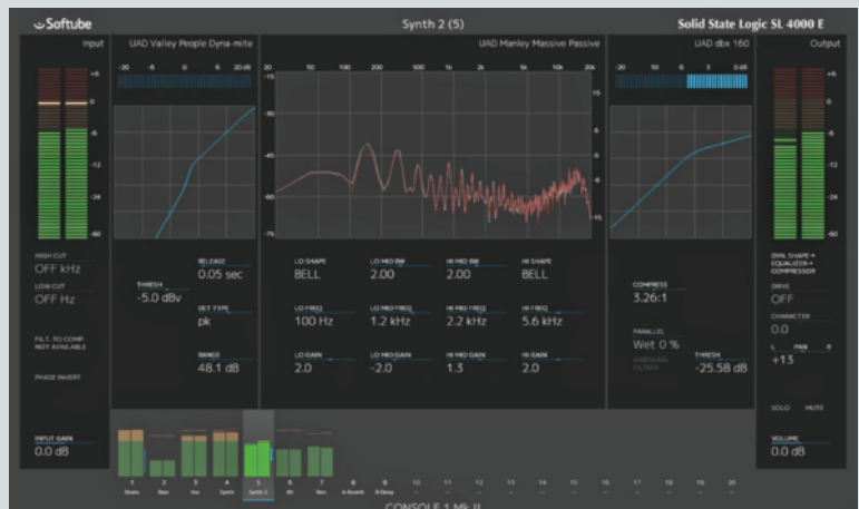
Three UAD plugin modules running in Console 1. In this case, all their parameters are available
