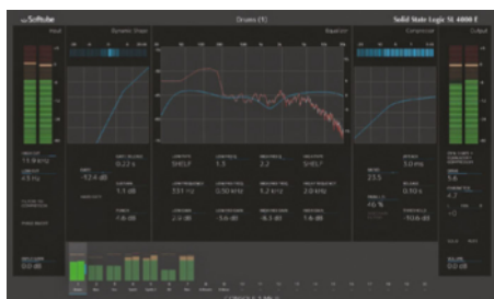
The On-Screen Display shows the loaded strip’s parameters, positionally matched to the hardware’s physical controls
