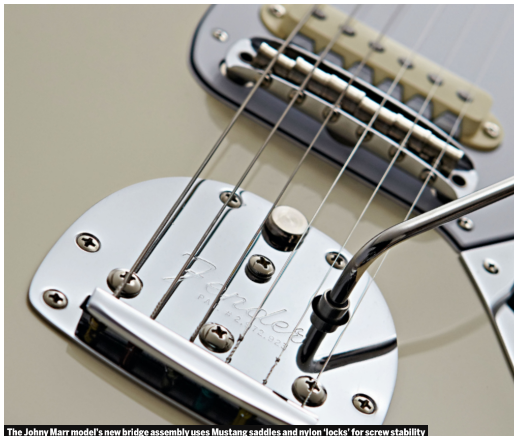
The Johnny Marr model's new bridge assembly uses Mustang saddles and nylon 'locks' for screw stability
